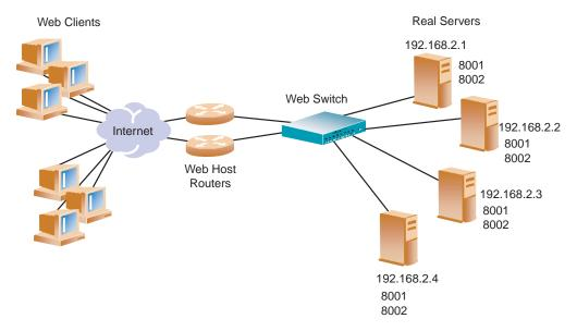
Figure 6-6 Basic Virtual Port to Real Port Mapping Configuration
